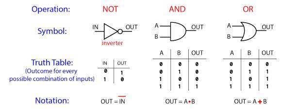
It turns out that any binary operator can be implemented by combining these 3 logic gates. For instance to implement the summation output described above, we can first breakdown the 4-bit output into the single bits and formulate each one in terms of the input bits. For example:
