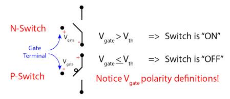
Replacing the resistor with this new switch should fix the problem (Threshold voltage of N-Switch and P-Switch is denoted by  $V_{th,N}$  and  $V_{th,P}$ , respectively):
