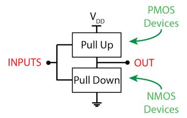
The job of the NMOS was to "pull down" the output to GND. Likewise, the job of the PMOS was to "pull up" the output to  $V_{DD}$ . They <u>never</u> do this at the same time! This is the underlying concept behind the logic gates we built from P- and N-switches as well. The following is the CMOS NOR gate:
