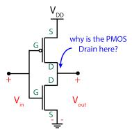
This circuit is directly derived from the switch-based inverter schematic. Pay close attention to the G, D, and S labels. Note  $V_{gate,N} = V_{in}$  and  $V_{gate,P} = V_{DD} - V_{in}$  and  $V_{out} = V_{DS,N}$ . Before we analyze the CMOS inverter, let's look at the first inverter we built using N-switch and resistance (called pseudo-NMOS inverter) shown below:
