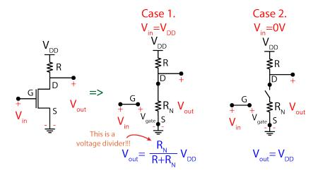
This figure revealed another issue of using only NMOS devices in addition to the static current in the ON state. The problem is that using transistor models with resistors, the output voltage is not 0V and it is a function of resistances and VDD. So for  $V_{out}$  to be low enough, R should be large again! However, in the CMOS inverter this issue does not exist:
