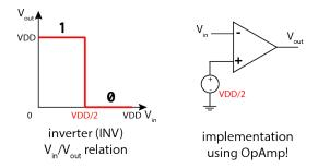
Although this works fine, we need around 10-20 transistors (explained later) to build a single opamp which is not affordable in terms of area and energy in practice! You will see how to build this gate using only two transistors!
