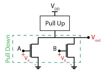
The pull down network (PDN) wants to short the output to GND if either  $V_A = V_{DD}$  or  $V_B = V_{DD}$  or both (check the condition of the NMOSs and see for yourself). We never want the Pull up network (PUN) to pull up the  $V_{out}$  to  $V_{DD}$  for any input combination that would pull  $V_{out}$  down to GND. Try this:
