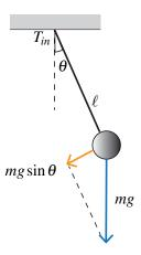
For state variables  $x_1 = \theta$  and  $x_2 = \omega$ , and input  $u = T_{in}$  the state-space equations for the pendulum are
