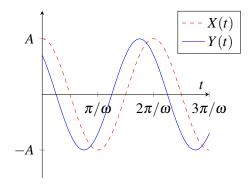
Here,  $\phi$  represents the **phase shift** of Y with respect to X. As can be seen, a positive phase shift moves the function to the left by that amount. In particular, notice that the sine and cosine functions are really the same sinusoid, with each just the other after a  $\pi/2$  radian phase shift in the appropriate direction.
