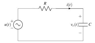
Let  $u(t) = V_0 \cos(\omega t + \frac{\pi}{2})$ . We are interested in finding how the voltage  $v_c(t)$  varies over time. Note that it is possible to solve this problem using differential equations, but we will now take advantage of phasors.<sup>4</sup>
