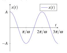
There are a couple properties of x(t) that are immediately apparent from the figure. We call the maximum value of x above the mean the **amplitude** (A), and the spacing between repetitions of the function the **period** ( $T = 2\pi/\omega$ ).
