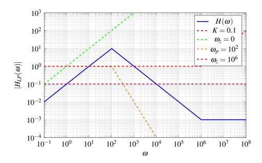
Since there is a zero at the origin, the plot initially starts with a slope of 1. There are no additional zeros or poles before  $\omega = 1$ , so we can approximate |H(1)| = K = 0.1. Then the double pole at  $\omega_p = 10^2$  provides a slope of -2 cancelling with the current slope of 1 making the overall slope after  $\omega_p$  equal to -1. Lastly, the zero at  $\omega_z = 10^6$  provides an additional slope of 1 making  $|H(\omega)|$  remains constant after  $\omega_z$ .
