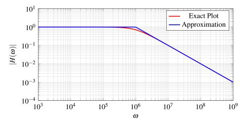
The Bode approximation matches the true plot very accurately. The largest approximation error in the straight-line plot occurs at the pole frequency  $\omega_p = \frac{1}{RC}$ . We approximate  $|H(\omega)|$  as 1 when in reality, it is equal to  $\frac{1}{\sqrt{2}}$ .
