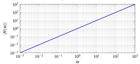
To plot a pole at the origin, notice that  $H(\omega) = \frac{1}{j\omega}$  has magnitude  $\omega$  and phase  $-90^{\circ}$ . If our transfer function has a pole at the origin, it will start off with a slope of -1.
