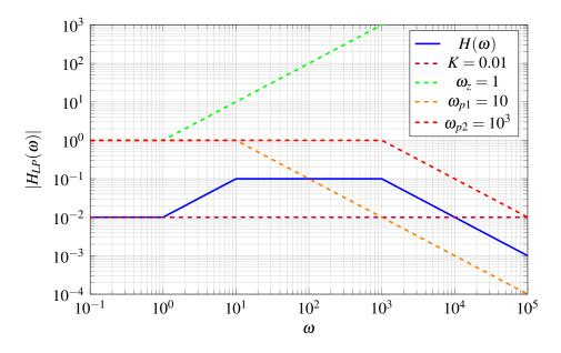
To provide an analysis for this Bode plot, we see that the plot starts off at K = 0.01. Then at  $\omega_z = 1$ , it starts rising with slope 1. When it hits the pole at  $\omega_{p1} = 10$ , the slope of 1 is cancelled out by the -1 slope that the pole provides. Then the Bode plot stays constant until  $\omega_{p2} = 10^3$  at which it drops off with a slope of 1. We've provided Bode plots of the individual terms to give you a sense of how we "add" Bode plots together.
