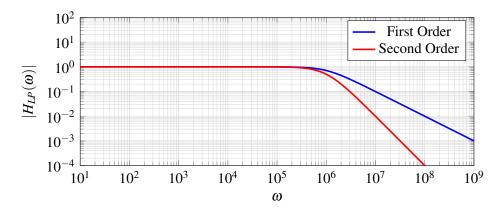
In fact, if we were to cascade even more low-pass filters, we approach an ideal low-pass filter in which
